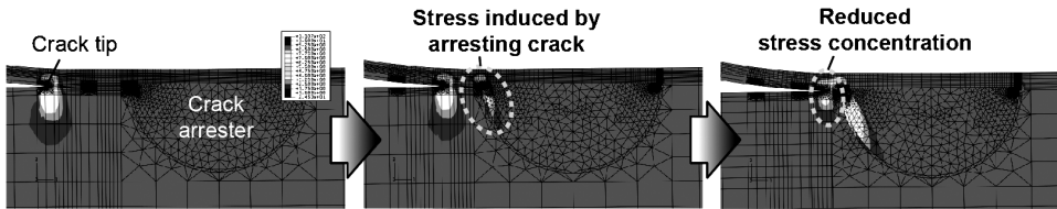
Figure 2. Distribution of normal stress in the vertical direction depending on crack tip position.
